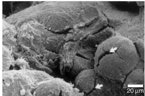
Figure 14 Electron micrograph of PLLA membrane with 11% plasticizer 14 days after implantation. The globular units of the membrane show the typical centrifugal fractures (arrows) of the degradation process.
